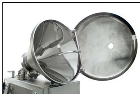
Hopper lid with filler opening can be tilted open
